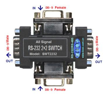
SWT2232 appearance for db-9 (female)/db-9 (male) dongle size, as shown in figure. The up db-9 (female) RS-232 and down db-9 (female) RS-232 can be directly plugged into computer's male db-9 RS - 232 serial ports. The left db-9 (male) and the right db-9 (male) ports are 2 switched RS-232 serial ports. SWT2232 needs no external power supply!
