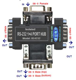
BS4232 appearance for db-9 (female)/db-9 (male) dongle size, as shown in figure. The up db-9 (female) RS-232 is directly plugged into computer's male db-9 RS - 232 serial port. The left db-9 (male), the right db-9 (male), and the down double db-9 (male) RS-232 ports are four isolated RS - 232 serial ports. BS4232 needs no external power supply!
